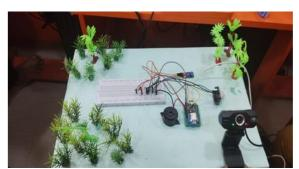
Figure 2 Prototype Setup of the Smart Wildlife Detection and Alerting System
