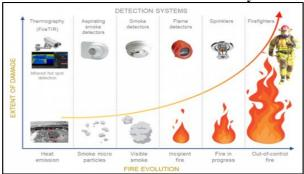
Figure 10 Stages of Fire: Detection and Warning Systems
