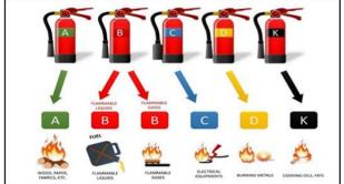
Figure 5 Fire extinguisher types and uses
