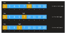
Figure 5 Step-by-Step Movement of Low and High Indices
