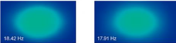
Figure 4. First mode shape of isolated RC slab under free vibration
