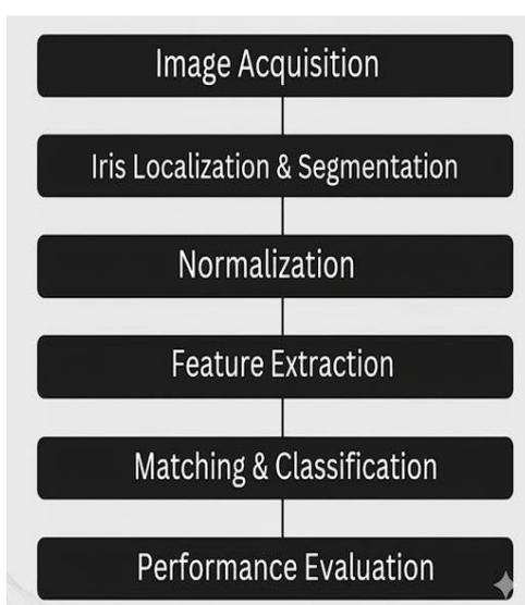
Figure 4 Workflow of the Iris Recognition System
