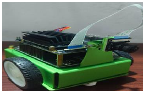
Figure 2 Assembled AI Pet Robot Prototype with Embedded Jetson Nano Platform
