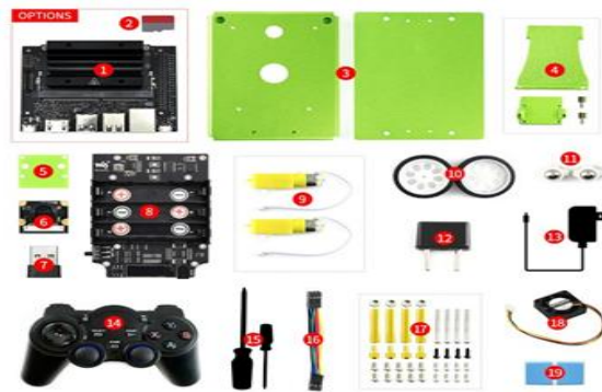
Figure 1 Hardware Components and Assembly Kit of the AI Pet Robot System
