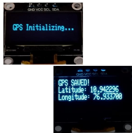
Figure 6 Presents the GPS initialization process, where the system searches for satellite signals and captures location coordinates once a stable fix is obtained. These coordinates are stored along with the complaint record.
