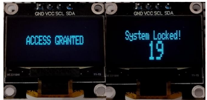
Figure 5 illustrates the access control behavior when the correct password is entered, the system displays “Access Granted”; otherwise, it locks for 30 seconds to prevent unauthorized attempts.
