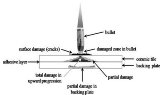
Figure 2 Damage zones in the ceramic tile, backing plate and a projectile (bullet)
