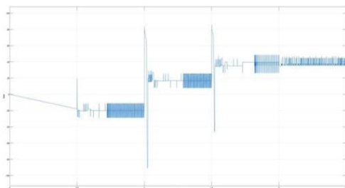
Figure 13 Motor Terminal Voltage V_m(t) Generated by The Mamdani FLC — MATLAB/Simulink Simulation. Three Distinct Average Voltage Levels Correspond to the Commanded Speed Set-Points; Superimposed PWM Ripple Confirms Correct H-Bridge
