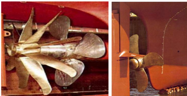
Fig.8. Grim Vane Wheel and Post-swirl Device
