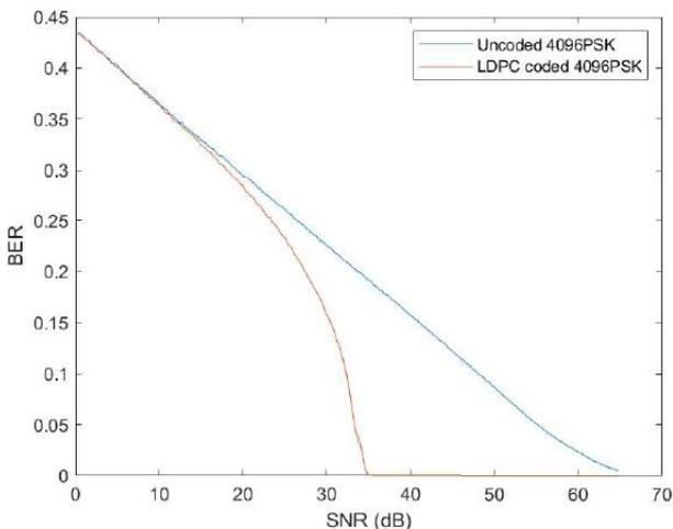
**Fig.10:Uncoded and LDPC coded 4096PSK**
