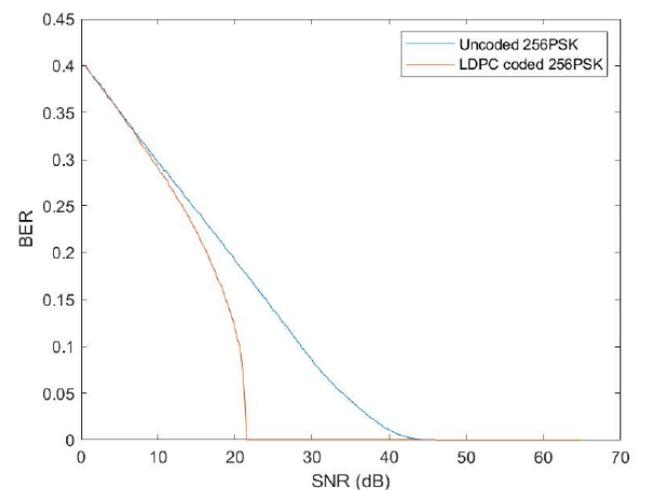
**Fig.7:Uncoded and LDPC coded 256PSK**
