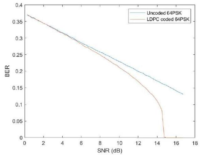
**Fig.5:Uncoded and LDPC coded 64PSK**
