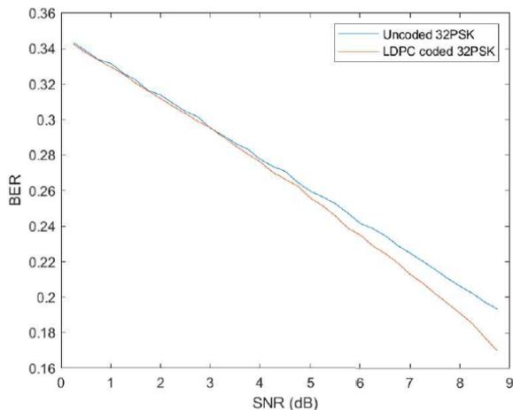
**Fig.4:Uncoded and LDPC coded 32PSK**
