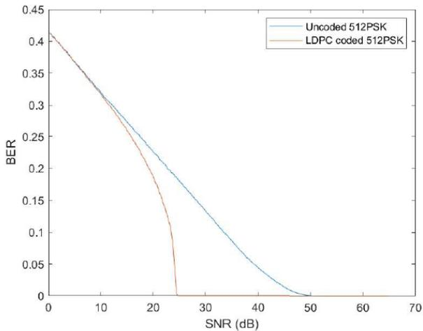
**Fig.8:Uncoded and LDPC coded 512PSK**
