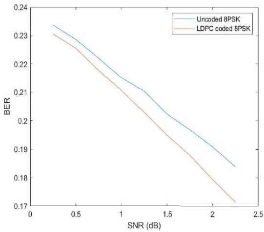
**Fig.2:Uncoded and LDPC coded 8PSK**
