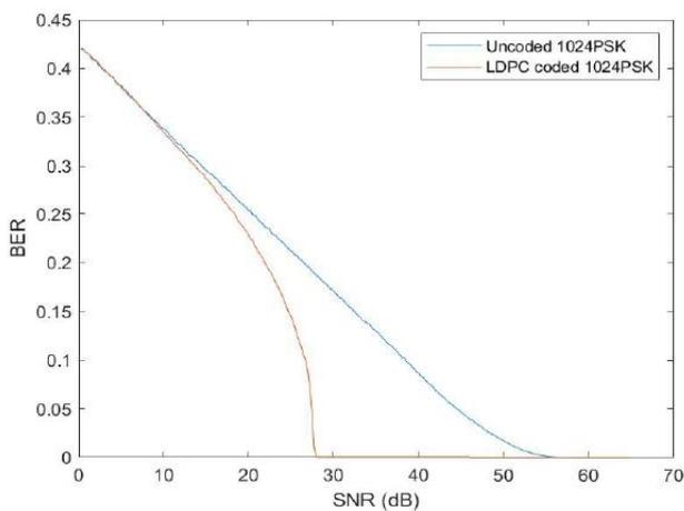
**Fig.9:Uncoded and LDPC coded 1024PSK**
