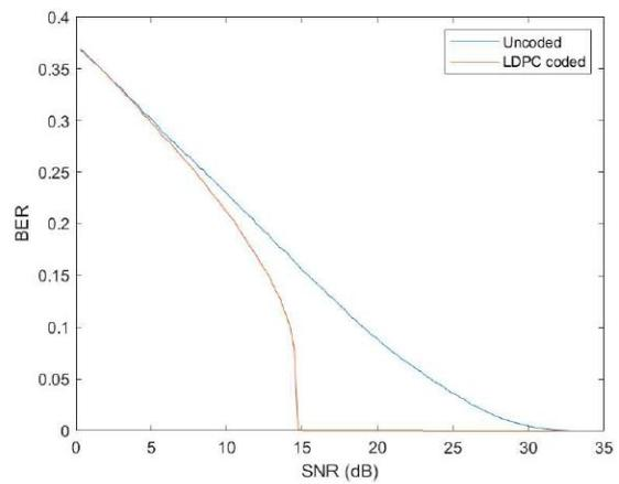
**Fig.6:Uncoded and LDPC coded 128PSK**
