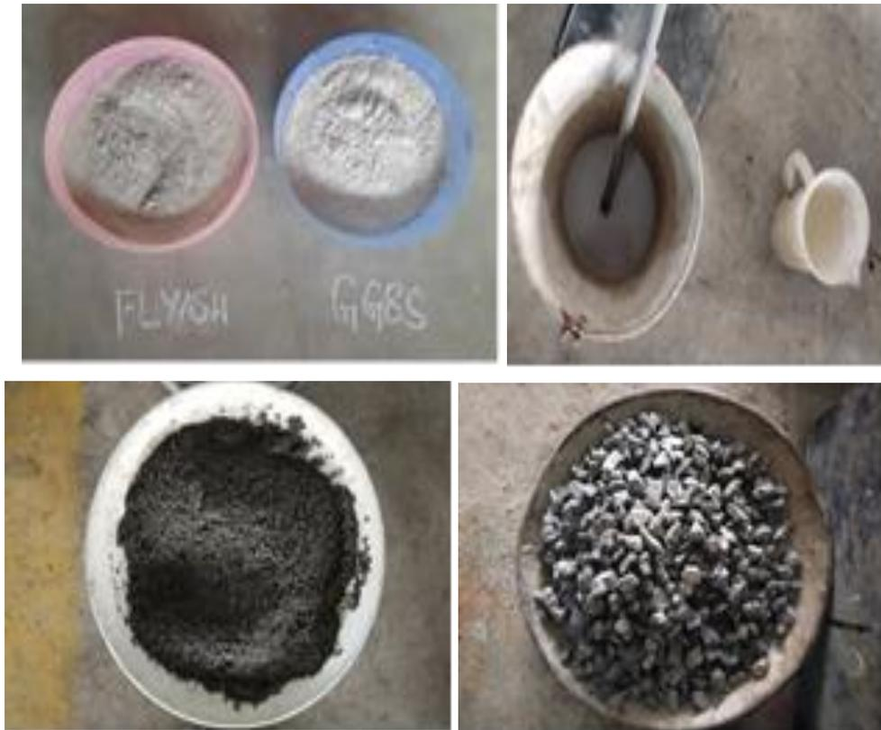
**Figure 1. Constituents of Geopolymer Concrete**
