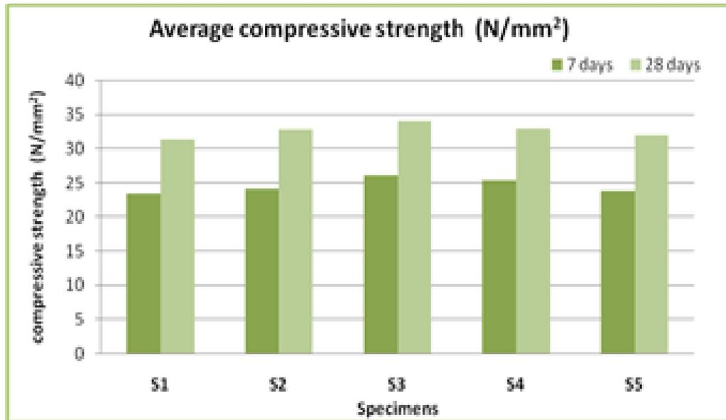
**Figure 2. Average compressive strength of geopolymer concrete**
