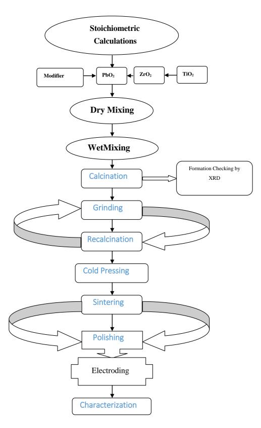
Fig.2. Flow Chart of Solid State Synthesis
