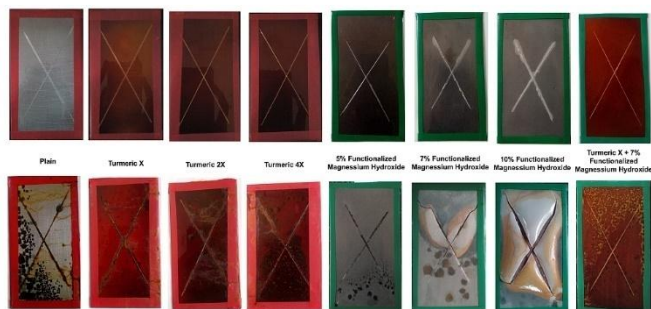
Fig. 8. Salt spray analysis of coating
