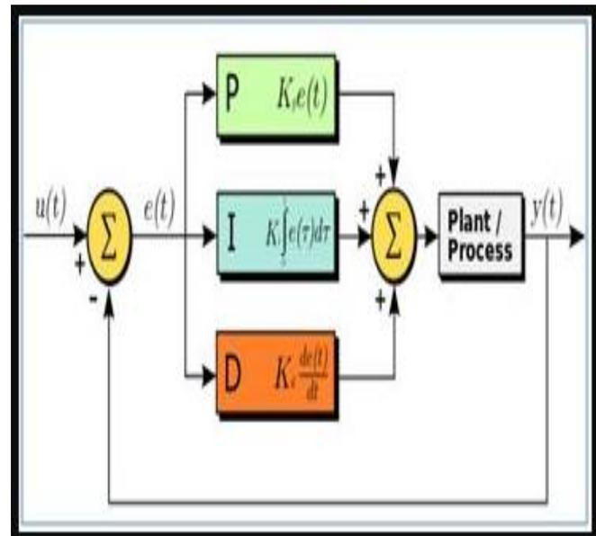
**Fig.1 Basic Diagram of PID Controller**
