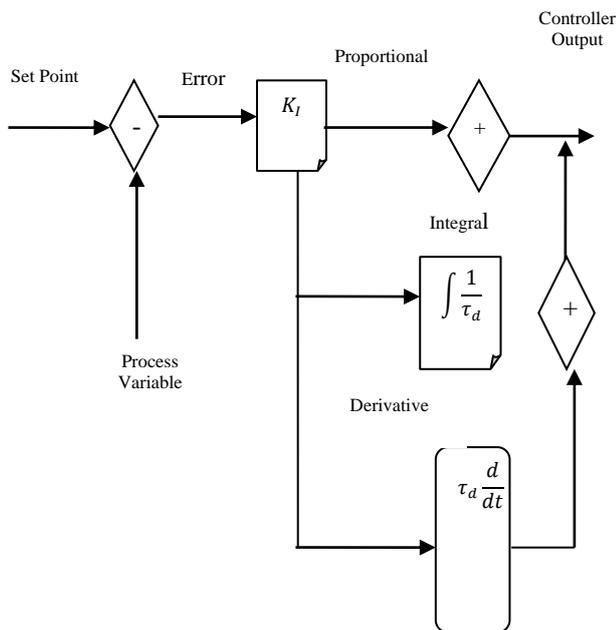
**Fig. 6 Basic Representation of PID Controller**
