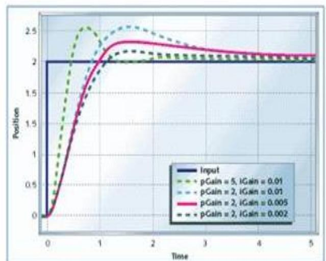
**Fig.5 PI Controller Response**
