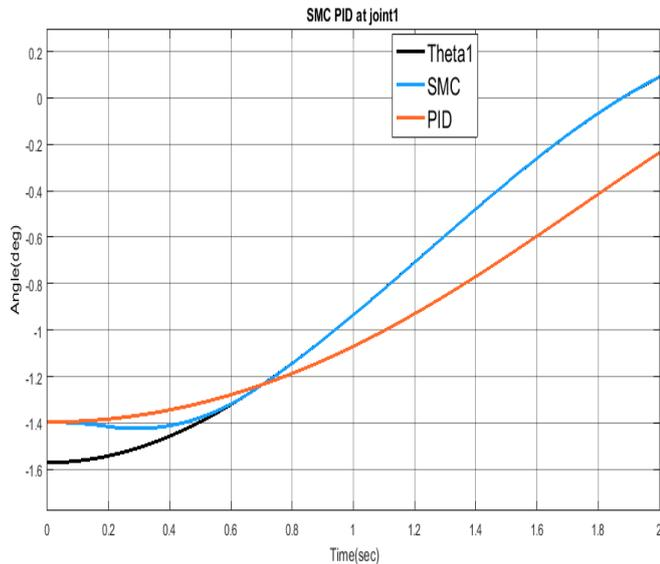
Fig. 10 Comparative results of SMC and PID at joint1
