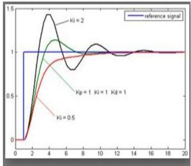
**Fig.7 PID Controller Response**
