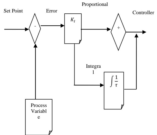
**Fig. 4 Design of PI Controller**
