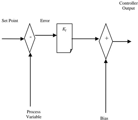
**Fig.2 Basic design of P-controller**
