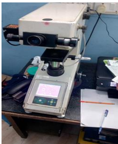
Fig.3. Microhardness testing setup
