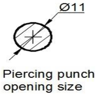
Fig. 5. Piercing punch opening size
