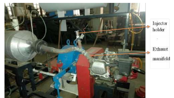
FIGURE 7. Pictorial View of Modified Exhaust
