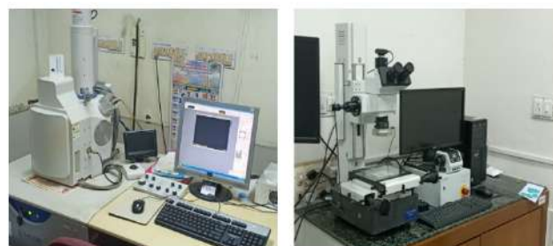
FIGURE 3. (a) Scanning Electron Microscope & (b) Digital Measuring Microscope
