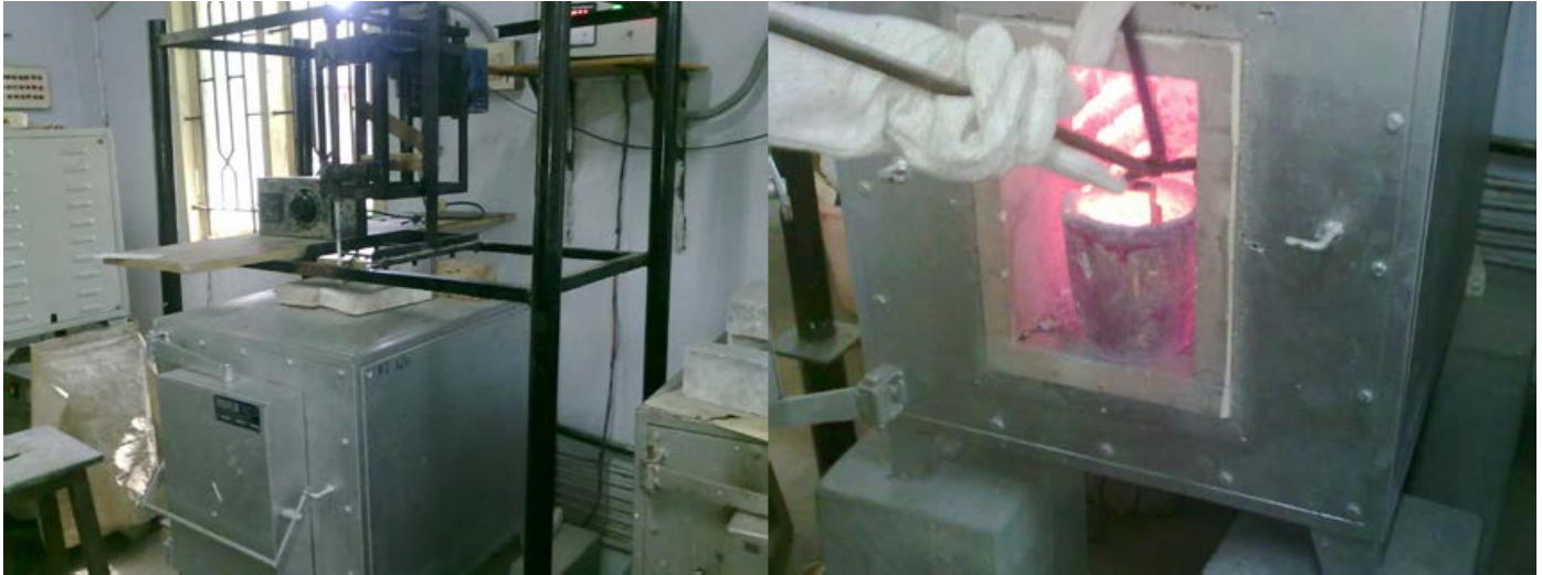
FIGURE 3. The experimental set up for production of hybrid MMC (Al6061-SiC-Al 2 O 3 ) composites
