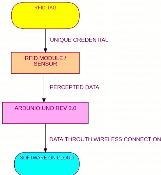
FIGURE 4. Hardware components flow diagram
