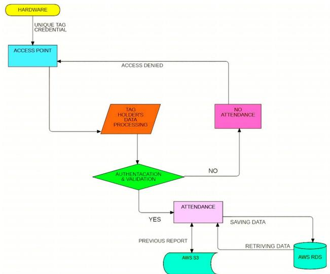
FIGURE 5. Software components flow diagram
