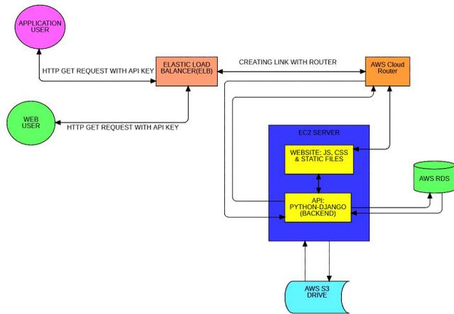
**FIGURE 6. Cloud components flow diagram**
