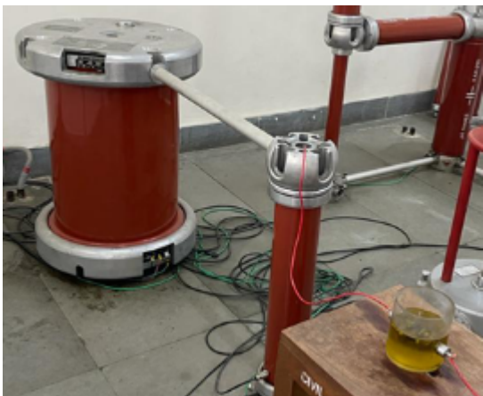
FIGURE 2. BDV test experimental setup.
