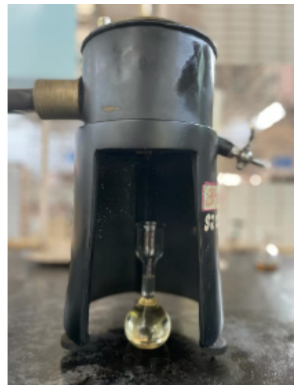
FIGURE 4. Test setup to measure viscosity.
