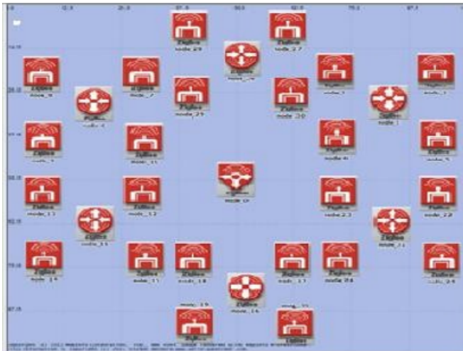
FIGURE 1. Static Node based IEEE 802.15.4 Cluster
