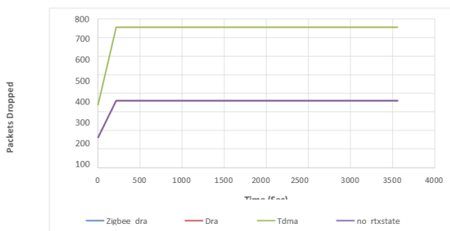
FIGURE 15. Packets Dropped in Static Networks
