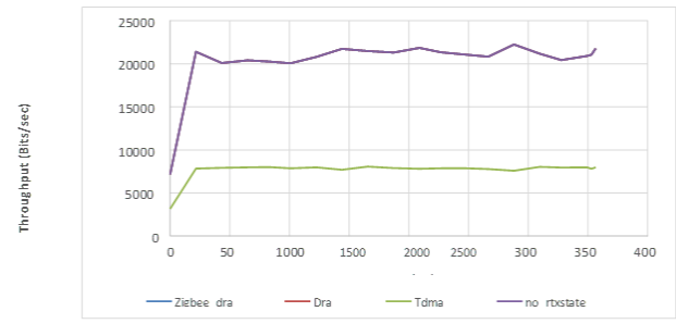
FIGURE 10. Throughput in Static Networks
