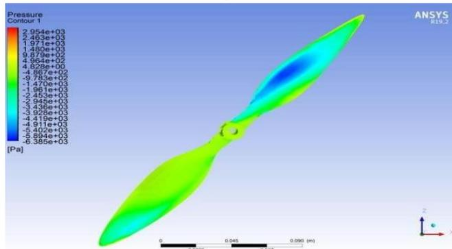
**Figure 6 Pressure Distribution in Bottom View**
