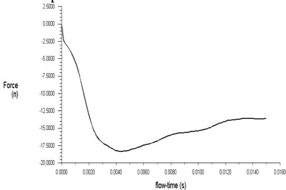
**Figure 17 Graph B/W Thrust Force and Flow Time**
