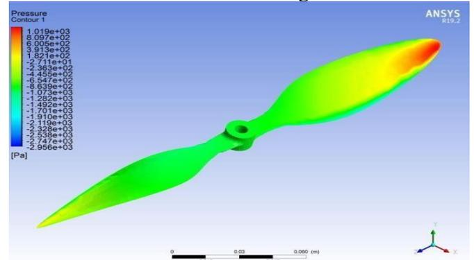
**Figure 7 Pressure Distribution in Isometric View**
