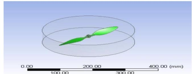
**Figure 1 Rotate Domain with 2 Blade Propeller**
