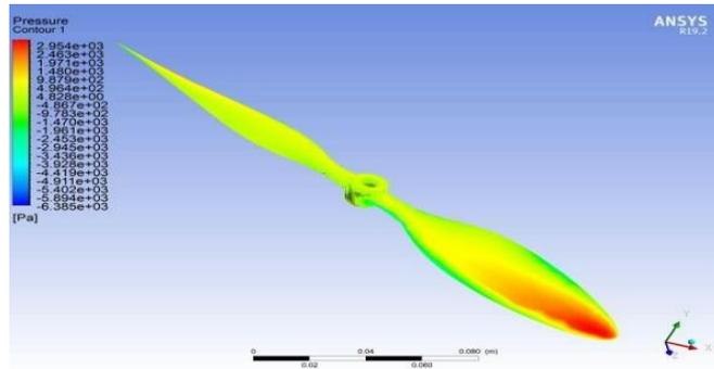
**Figure 5 Pressure Distribution in Isometric View**
