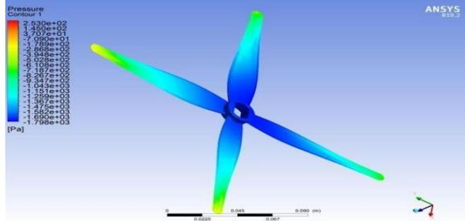
Figure 13 Pressure Distribution in Isometric View
