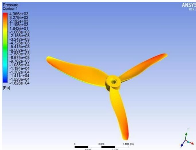
**Figure 9 Pressure Distribution in Isometric View**
