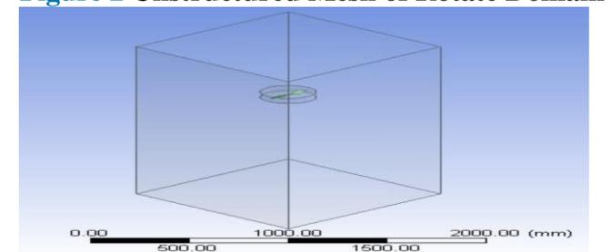
**Figure 3 Static Domain with Rotate Domain Inside**
