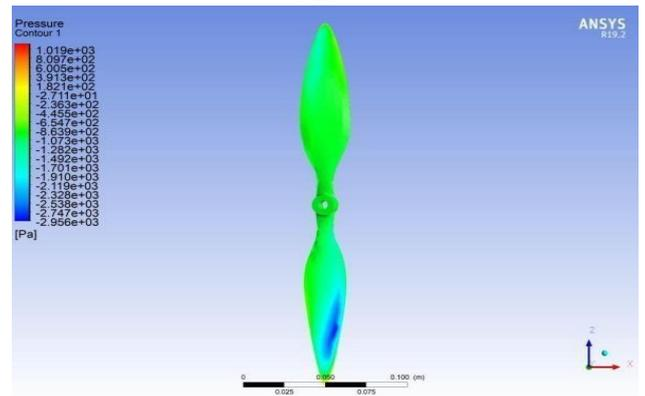
**Figure 8 Pressure Distribution in Bottom View**
