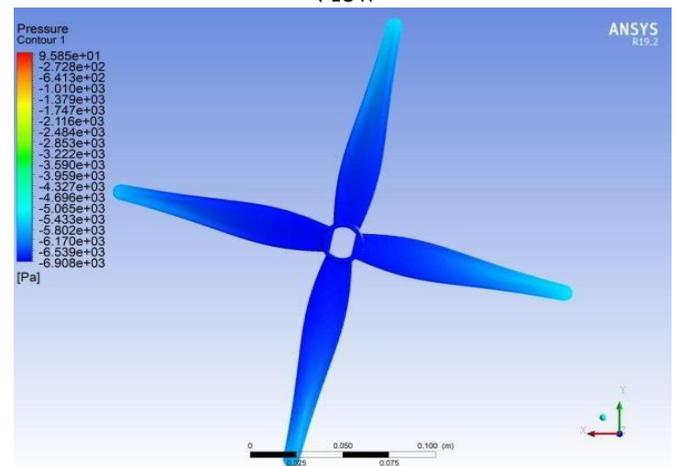
Figure 16 Pressure Distribution in Bottom View
