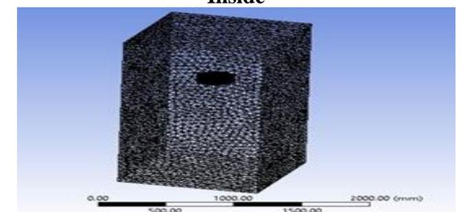
**Figure 4 Unstructured Mesh of Static Domain**
