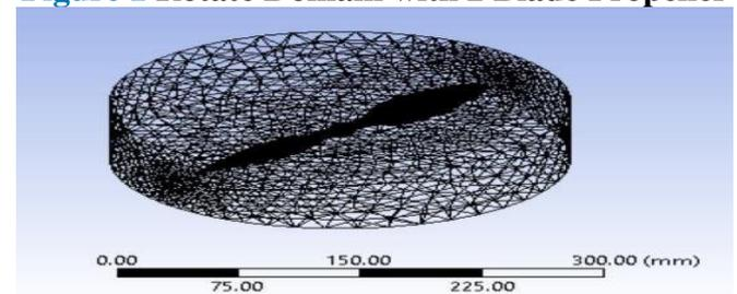
**Figure 2 Unstructured Mesh of Rotate Domain**
