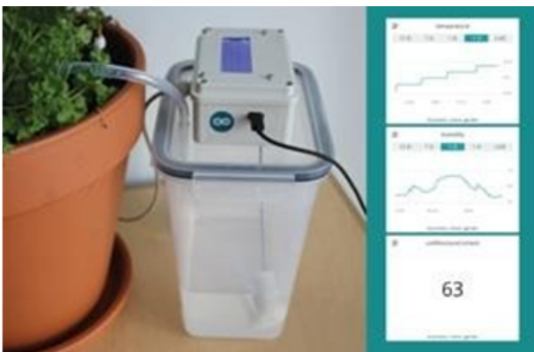
FIGURE 9. Pumping water automatically after reading the values
