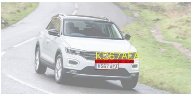
FIGURE 12. Example using a license plate in foggy conditions with 50% visibility.
