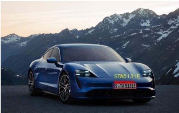
FIGURE 11. Example using license plate with similarly shaped characters (5 and S).
