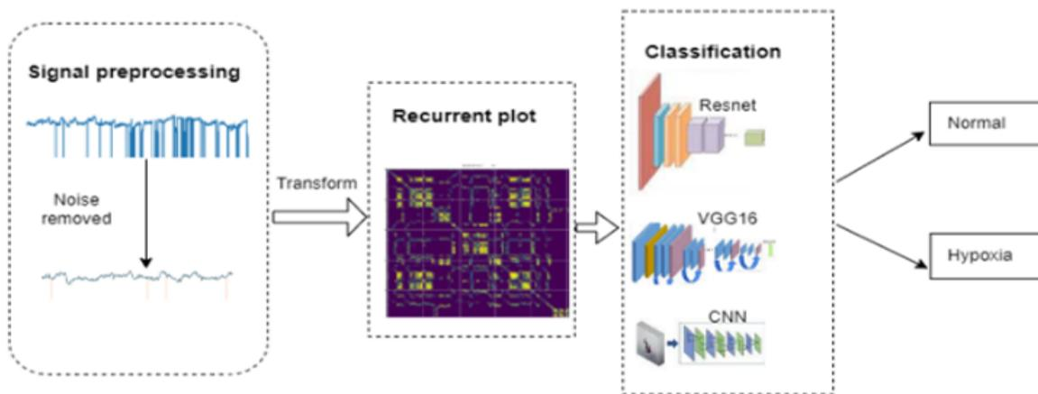
**FIGURE 2. Architecture of the CTG classification system**
