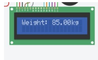
FIGURE 19. The LCD output when the device displays the user's weight.
