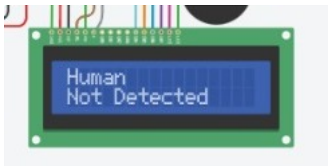
FIGURE 21. The output of the LCD is when the device displays the detection of humans.
