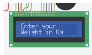
FIGURE 18. The output of the LCD is when the device asks the user to enter their weight.
