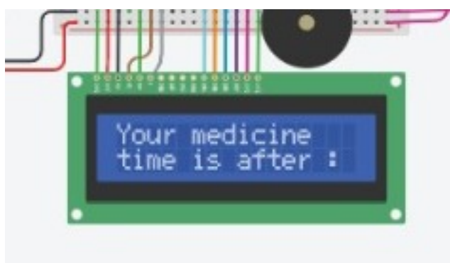
FIGURE 23. The output of the LCD is when the device displays the remainder of the time to take medicine.
