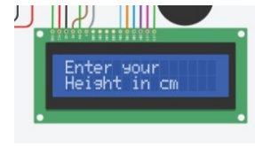
FIGURE 16. The output of the LCD is when the device asks the user to enter their height.
