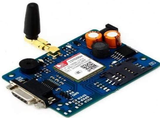
**FIGURE 5. GSM Module**
