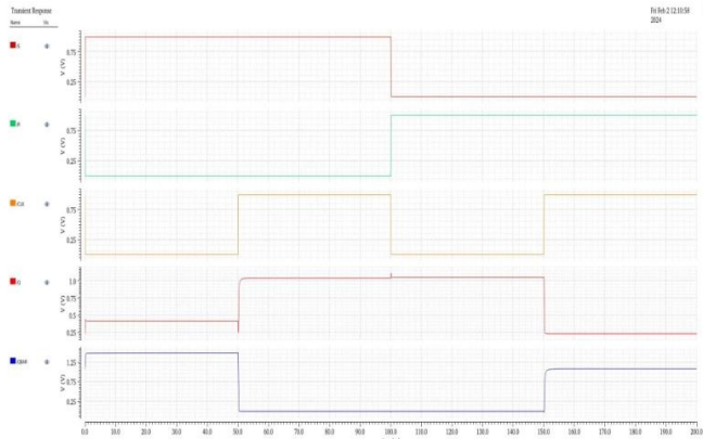
Figure 6 Simulation Result of ONOFIC SR Flip Flop
