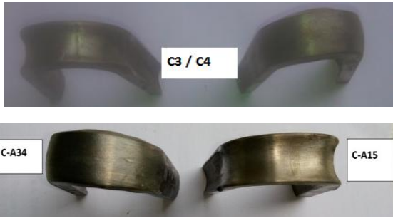
Fig. 6 SA 210 Gr C Specimens After Face & Root Bend Testing
