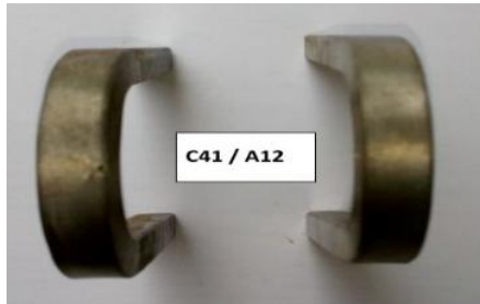
Fig. 7 SA 213 T12 Specimens After Face & Root Bend Testing
