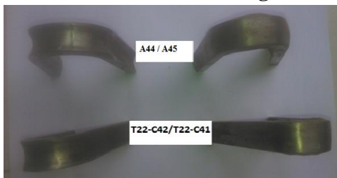
Fig. 7 SA 213 T12 Specimens After Face & Root Bend Testing
