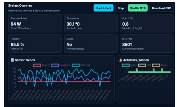
Figure 4 System Overview with temperature, humidity, LDR, motion, and power
