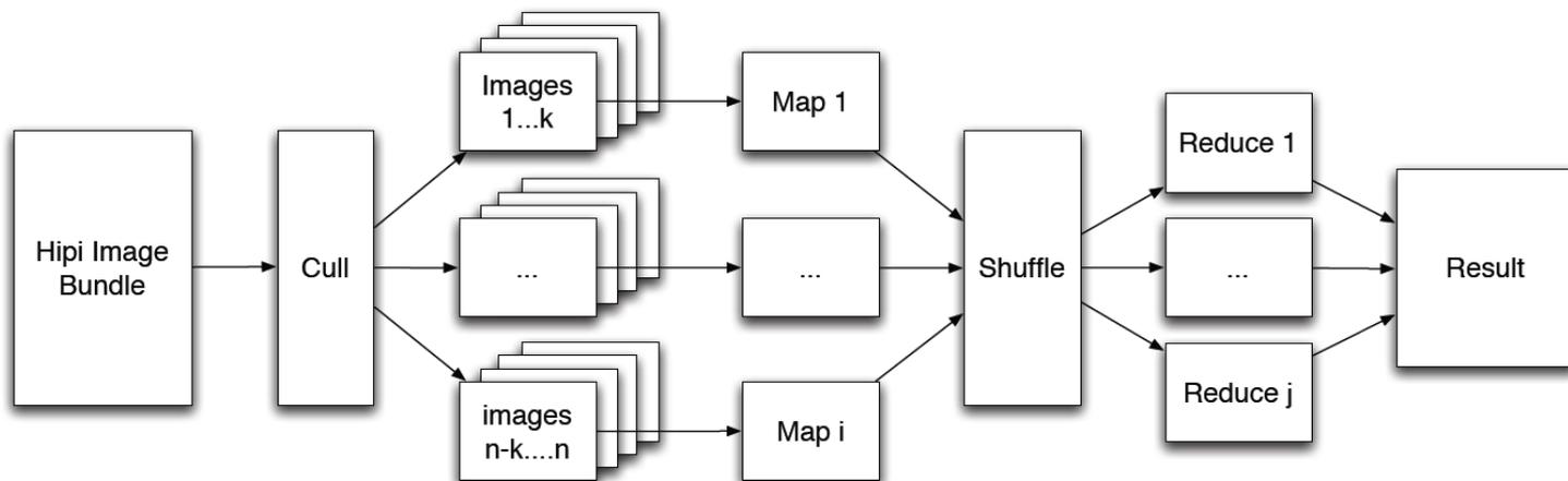
**Fig 3: Hadoop Image processing Interface.**
