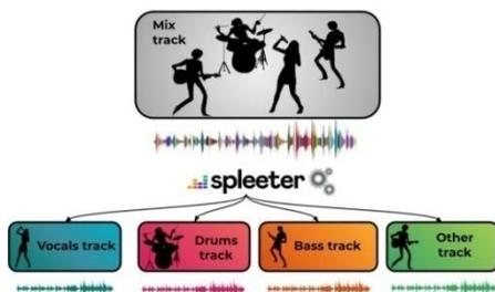
**Fig.1. Source separation representation**
