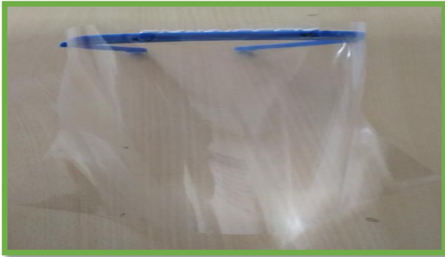
Fig.5 Face shield frame printed with our 3D printer
